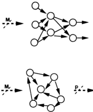
Diagram of sequential (top) and recurrent (bottom) neural networks, from Siegelmann 1999
